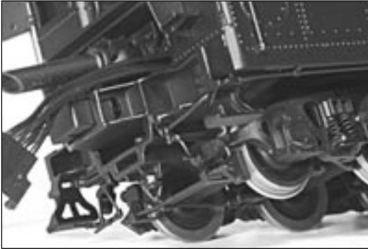
The photograph to the left shows the drawbar release hanging down under the operational buffer assembly. The prototypical double drawbar inserts into the two slots just above the release.
